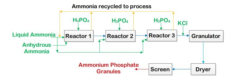
**Figure:** Manufacturing of Ammonium Phosphate
